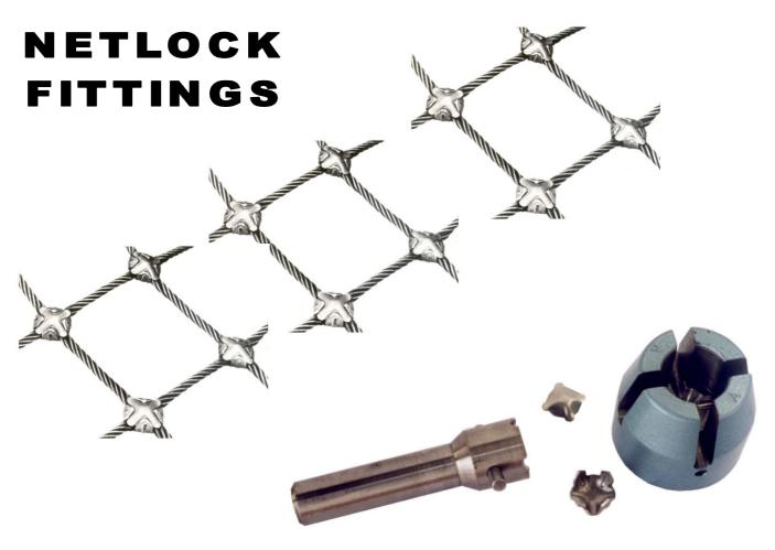
The **SAHM SPLICE** - **NETLOCK** fittings system is the simple method for producing nets in materials such as Synthetic fibre and Steel wire ropes. Only a hammer and **NETLOCK PUNCH** are required to effect secure joints. Fittings are available in Carbon steel, Stainless steel and Aluminium alloy.
